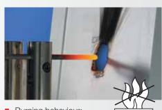
Burning behaviour: 750°C Glow wire test according to IEC 60 695-2-11: 750 °C, flame-retardant, self-extinguishing
